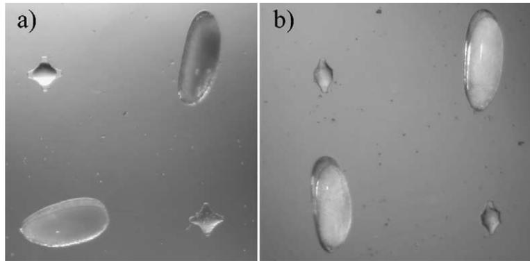
Fig. 5. Close-up images of (a) oil-covered  $200\ \mu\text{m} \times 200\ \mu\text{m}$  cross-shaped; and (b)  $200\ \mu\text{m} \times 100\ \mu\text{m}$  truncated cross-shaped pads with and without immobilized embryos. An example of an immobilization site only partly covered by the oil film can be discerned in the upper left corner of (a).
