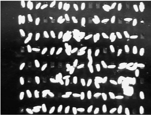
Fig. 3. Embryos immobilized at a sample patterned with an array of rectangular 250\ \mu\text{m} \times 400\ \mu\text{m} sized immobilization sites. A substantial amount of clustering is observed.
