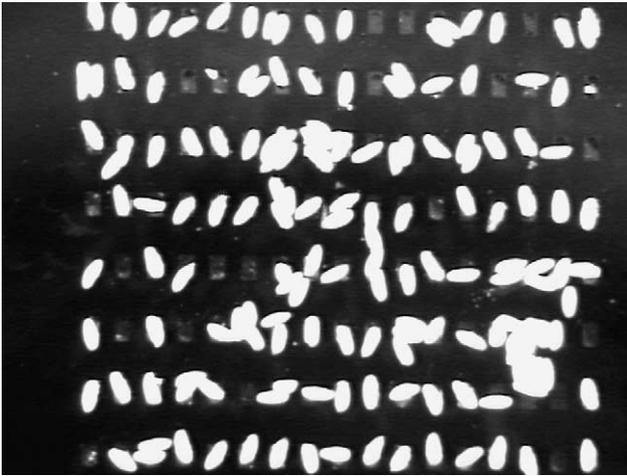
Fig. 3. Embryos immobilized at a sample patterned with an array of rectangular  $250\ \mu\text{m} \times 400\ \mu\text{m}$  sized immobilization sites. A substantial amount of clustering is observed.
