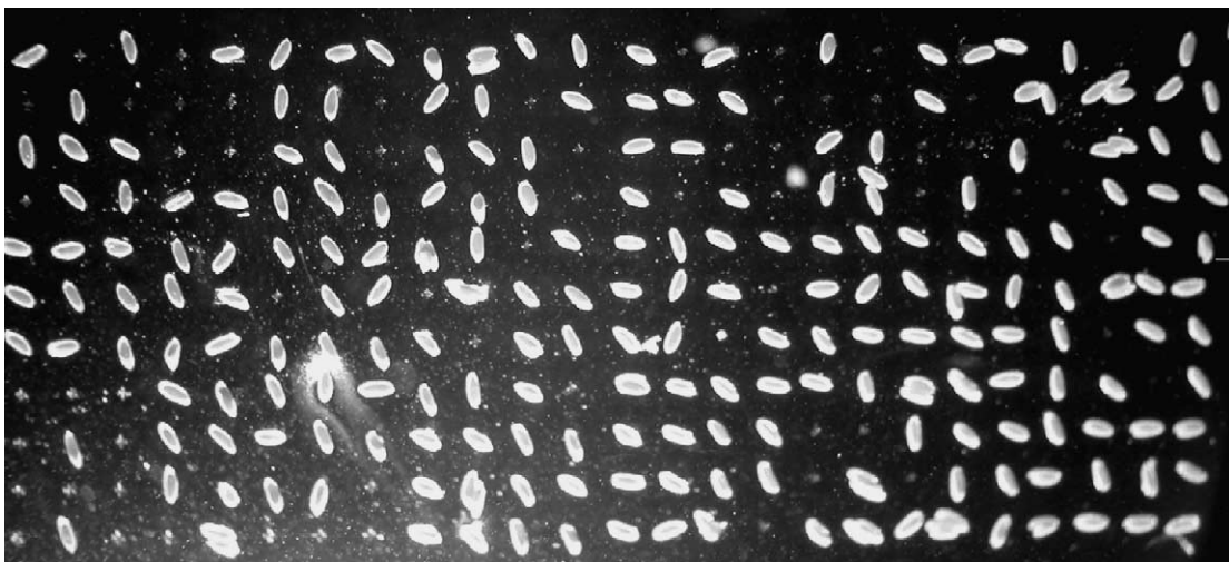
Fig. 4. An image of embryos immobilized at a sample patterned array with 200\ \mu\text{m} \times 200\ \mu\text{m} cross-shaped and 200\ \mu\text{m} \times 100\ \mu\text{m} truncated cross-shaped sites with 800\ \mu\text{m} \times 800\ \mu\text{m} pitch. The clustering is reduced substantially.
