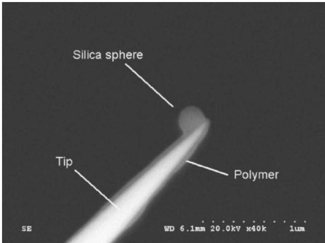
Fig. 2. Attachment of lumophores at the probe tip, where 200-nm-sized silica sphere covered with CdSe/ZnS QDs is attached to a scanning tip (From [5]. Reprinted with permission).
