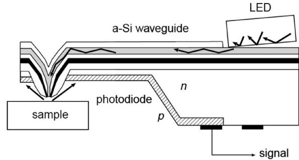
Fig. 5. Coupling of LED to a scanning probe integrated with waveguide, aperture, and photodiode (From [21]. Reprinted with permission).
