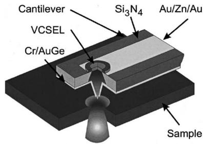
Fig. 4. Integration of laser diodes, such as VCSEL, with micromachined cantilevers (From [20]. Reprinted with permission).
