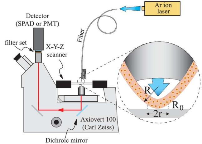
Fig. 3. Fiber-based excitation of the lumophores at the tip and the specimens under investigation (From [9]. Copyright (c) 2003, Blackwell Publishing Ltd. Reprinted with permission). CdSe QDs were attached at a fiber tip and excited by an Ar ion laser. Emission from the particles is used to excite lumophores at the sample for imaging.
