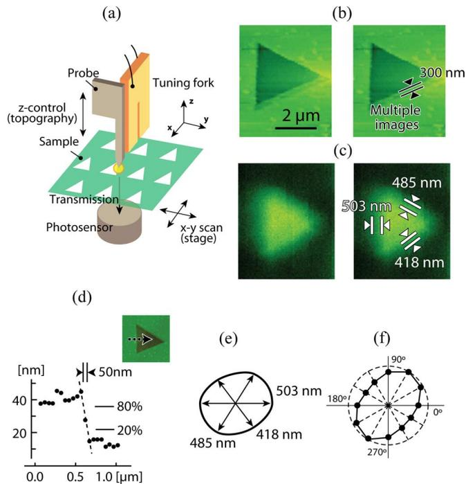
Fig. 9. Near-field scanning nanophotonic microscopy. (a) Schematics of the experimental setup. (b) Topographic images. Multiple images of an edge are visible. (c) Optical images. Directional dependence of the resolution was identified. (d) Topographic profile of an edge of a triangle pattern. (e) Nano-LED shape is estimated from the optical image. (f) Polarization of the Nano-LED measured with a rotating polarizer.
