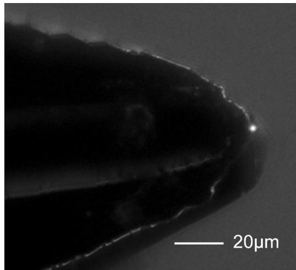
Fig. 7. Electroluminescence from QDs trapped to the nanogap at the probe tip.
