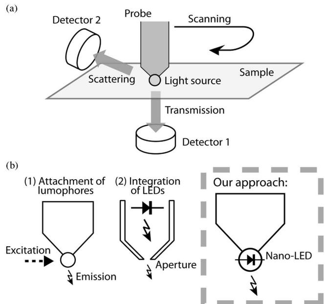
Fig. 1. Overview of the near-field scanning nanophotonic microscopy. (a) Schematic of a standard NSOM. (b) Integration of miniature light sources on the probe. Two conventional approaches include: (1) attachment of fluorescent light sources at the tip and (2) integration of an LED and an aperture. Our method is shown in (3) creation of Nano-LED at the tip.
