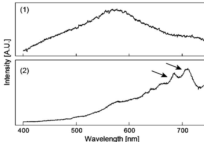
Fig. 8. Emission spectra of the two types of Nano-LEDs: (1) silicon-dioxide-based LED. (2) QD attached LED. Small additional emission peaks are found in (2), while both (1) and (2) have a common broad peak around 580 nm.
