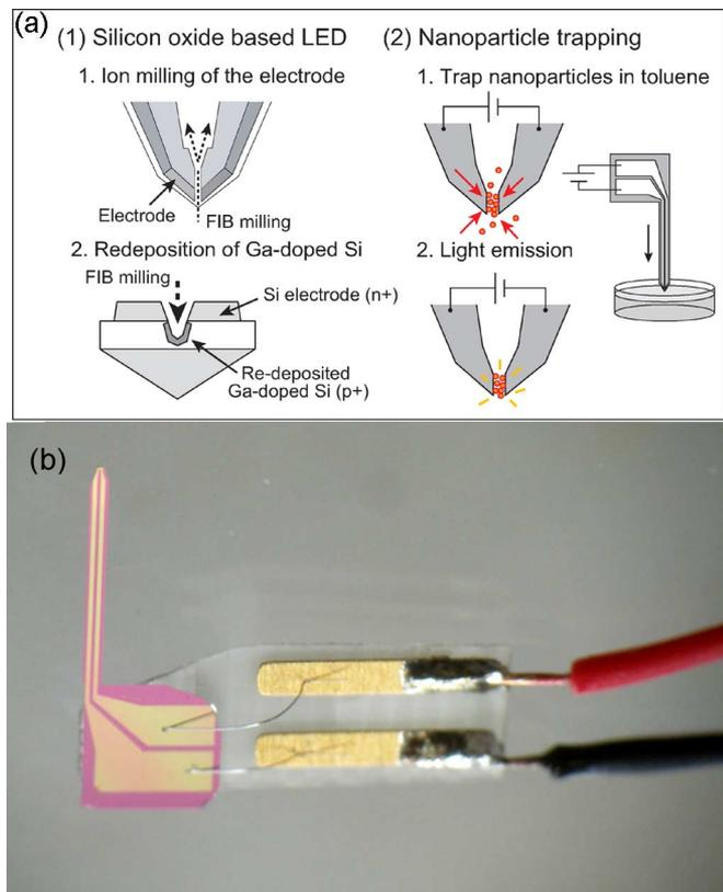
Fig. 6. Design and fabrication of Nano-LEDs on the probe tip. (a) Two methods of Nano-LED integration. (1) Silicon probe is directly doped with FIB and (2) CdSe nanoparticles are trapped at the FIB-created nanogap. (b) Photograph of the nanophotonic scanning probe.
