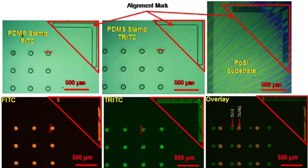
**Fig. 5** *Top, left to right:* PDMS stamp used to stamp FITC rabbit IgG antibodies; PDMS stamped used to stamp TRITC rabbit IgG antibodies; nanoporous silica substrate. All three have corresponding alignment markings to facilitate accurate stamping. *Bottom, left to*
