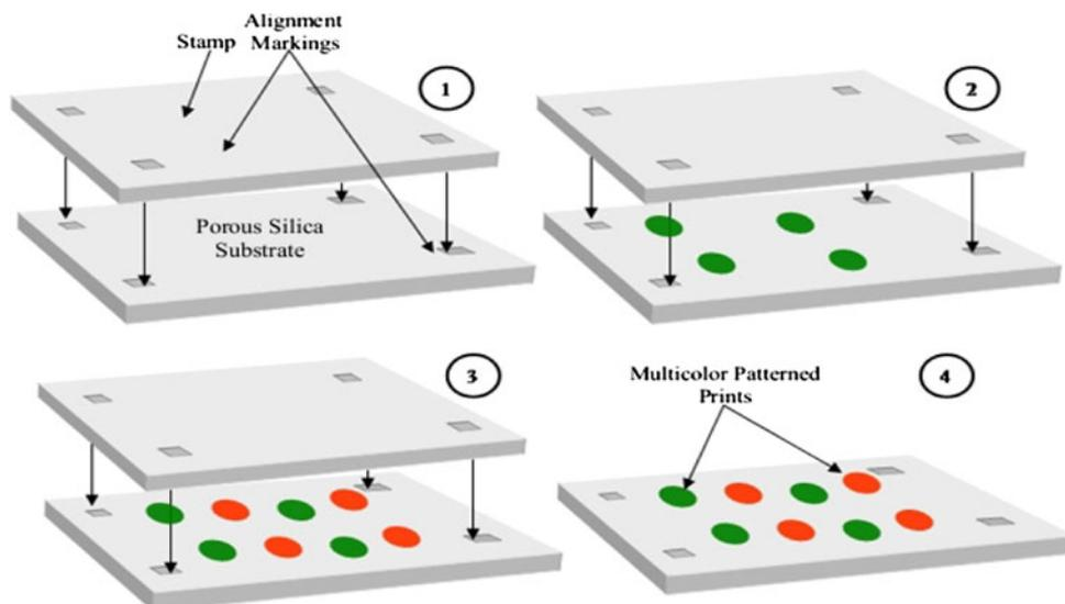
**Fig. 4** **a** Theoretical molecular structure of a single sandwich ELISA. The ultimate binding of the detecting secondary antibody, tagged by a fluorophore, enables optical detection when excited by a light source. **b** Schematic of the microcontact sandwich ELISA process. The capture antibody is microcontact printed onto the nanoporous silica substrate surface. Subsequent pipetting of specific antibodies builds and completes the sandwich ELISA
