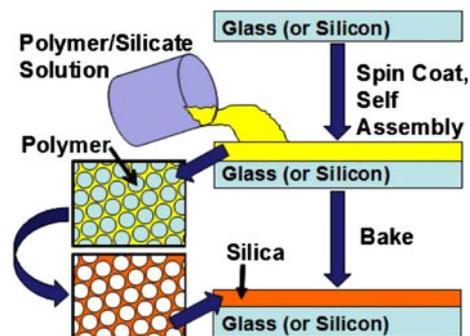
**Fig. 1** Schematic of the fabrication of nanoporous silica substrates (Hu et al. 2009)
