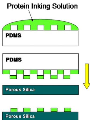
**Fig. 2** Schematic of the microcontact printing process
