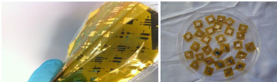
**FIGURE 5.** Images of flexible pressure sensors on kapton film.
