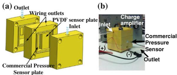
**FIGURE 2.** Flow chamber assembly for sensor measurements. (a) Schematic showing chamber with air flow through the system; and (b) actual photograph of chamber in the testing setup.
