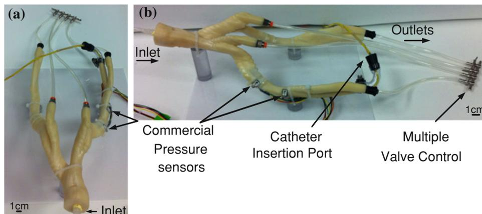
**FIGURE 3.** Vascular testing model with integrated sensor.
