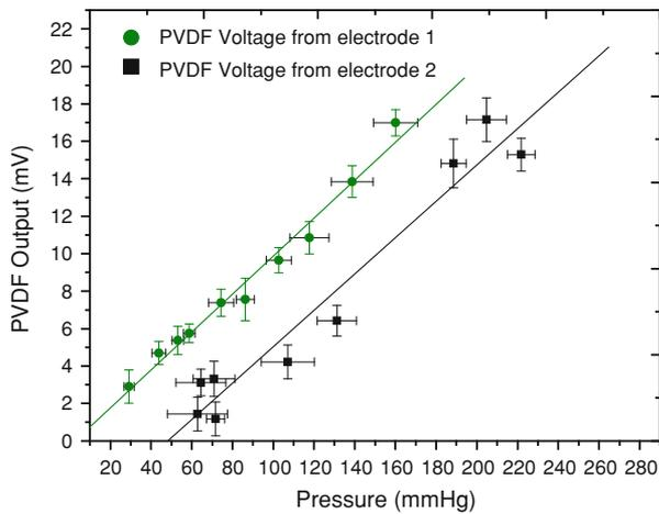
**FIGURE 7. The flexible-PVDF sensor response versus the chamber pressure for two independent top electrodes. Slope of the graphs indicate reliable performance from the two electrodes with different zero errors and a high sensitivity of  $99 \mu\text{V}/\text{mmHg}$ .**
