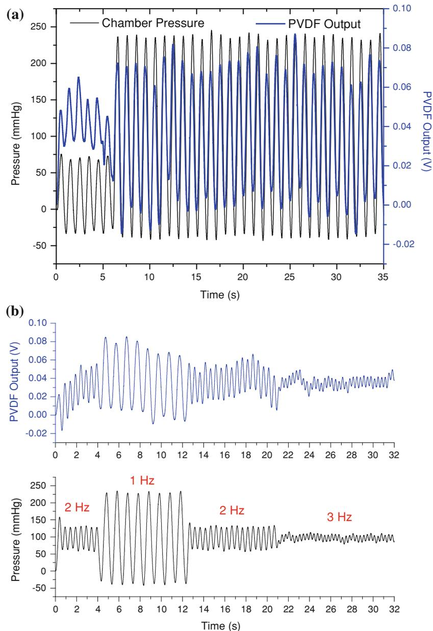
**FIGURE 6.** Comparison of real-time pressure measurements using PVDF thin-film sensor (blue curve) and Freescale pressure sensor (black curve) as a function of the (a) ambient pressure change in chamber; and (b) chamber pressure frequency.
