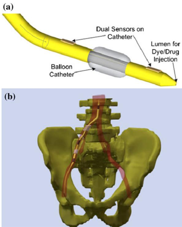
**FIGURE 1.** Concept of smart catheter with integrated pressure sensors. (a) Schematic showing the desired placement of PVDF based thin film pressure sensors on catheter; and (b) schematic showing placement of a two-balloon catheter in iliac artery with multiple pressure sensors on either side of the balloon.
