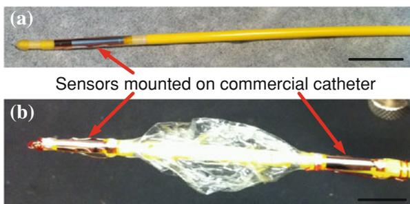
**FIGURE 4.** (a) Photographs showing PVDF pressure sensors mounted on catheter; and (b) on either side of balloon. Scale bars: 1 cm.
