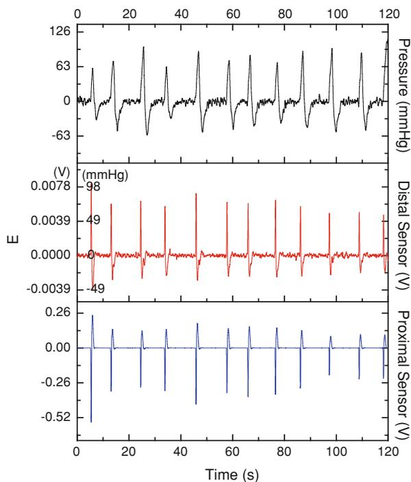
**FIGURE 8. Comparison of the proximal (closer to catheter tip) and distal (away from catheter tip) PVDF sensors against the fluid-pressure inside the vascular model. It shows shorter response times of PVDF sensors (0.26 s) compared to the commercial pressure sensor (1.30 s).**
