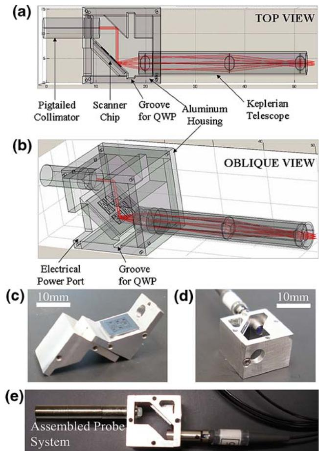
**Fig. 3** The handheld MEMS probe package. (a) Schematic top view of layout, depicting optical components and light path, (b) Oblique view of the MEMS packaging scheme, (c) Photograph of the two blocks forming part of the package, with microscanner chip mounted, (d) Assembled package with pigtailed collimator inserted into the input optical port, (e) Full mechanical probe assembly (top and bottom cover plates of the package not shown in images)
