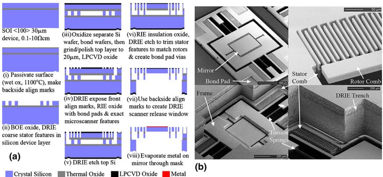
**Fig. 1** High-reflectivity two-axis vertical combdrive microscanners. **(a)** Process flow for device fabrication, **(b)** Scanning electron micrographs (SEM) of fabricated microscanners depicting mirror and
