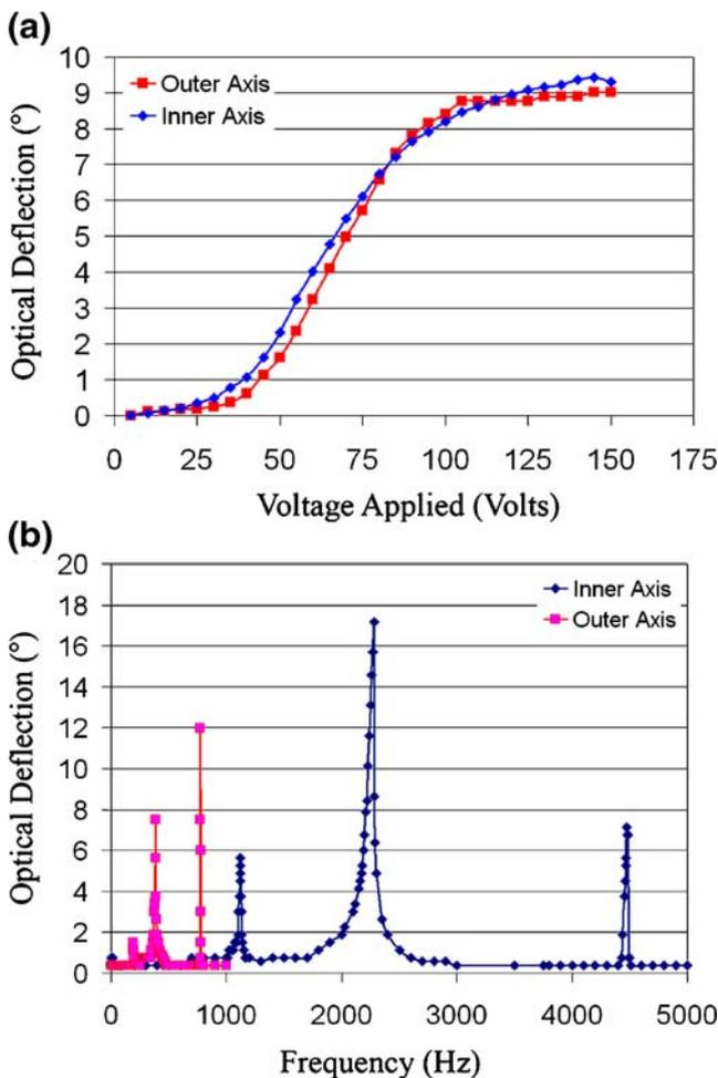
**Fig. 2** Microscanner operating characteristics. (a) Single-sided static voltage deflection characteristics, (b) Frequency-dependent optical deflection. Applied voltage,  $V = 18.0 + 9.0 \sin(2\pi ft)$  volts
