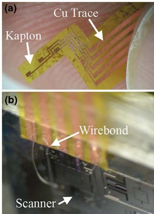
**Fig. 4** Flexible electrical routing circuit. (a) Photograph of copper electrical traces fabricated on flexible Kapton substrate, (b) Photograph of wire-bonding connections made between the flexible routing traces and the silicon stator layer on microscanner chip
