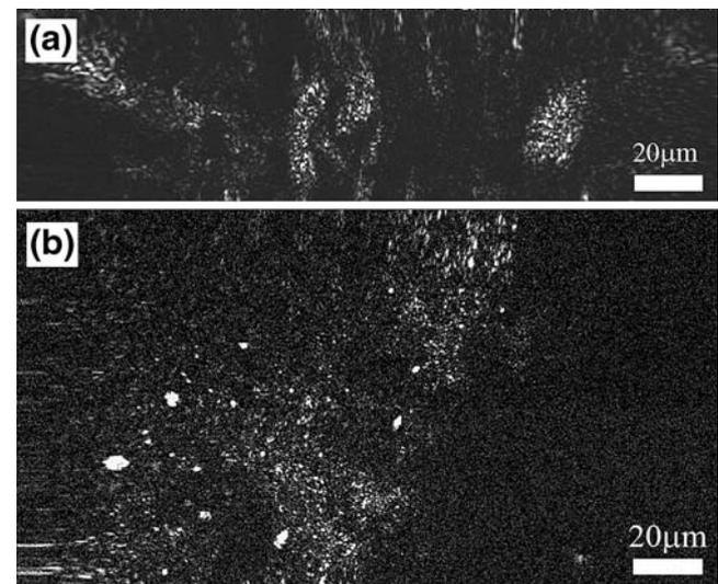
**Fig. 7** MEMS Confocal images of biological samples. (a) *In vitro* oral porcine tissue treated with acetic acid, obtained using single-sided scan on the outer microscanner axis. Field of view is  $200 \mu m \times 55 \mu m$  approximately; (b) *In vivo* human fingernail. Cell nuclei and cell borders are visible. Field of view is  $200 \mu m \times 110 \mu m$ . Videos of samples were acquired at 3.5–5.0 frames per second
