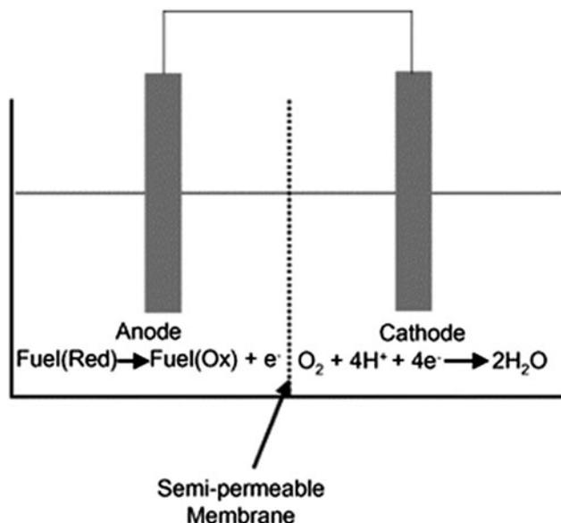
**Figure 5.** Schematic of a basic biofuel cell consisting an anode, cathode, and a semipermeable membrane.<sup>79</sup>
