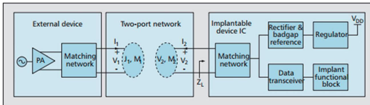
**Figure 3.** Block diagram showing the various components of a wireless transmission system utilizing RF antennas for energy transfer. Key components include the matching network, rectifier, regulator, and band gap reference. Source: Ref. 52.
