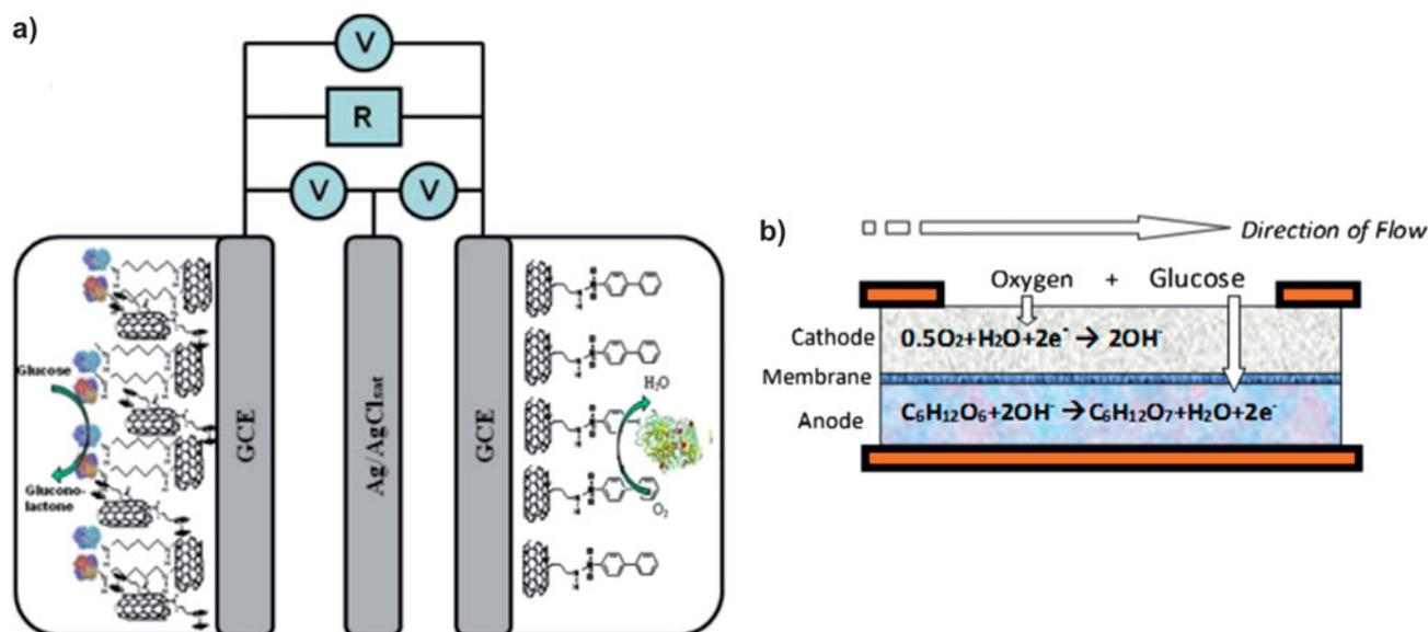
**Figure 6.** (a) Schematic of enzymatic biofuel cell demonstrated by Stolarczyk et al. showing mechanism of oxidation at the biological – gold-coated electrode (GCE) anode and reduction at the cathode<sup>80</sup>; and (b) schematic of AGFC showing mechanism of selective glucose oxidation by oxygen depletion at the cathode. Source: Ref. 103.
