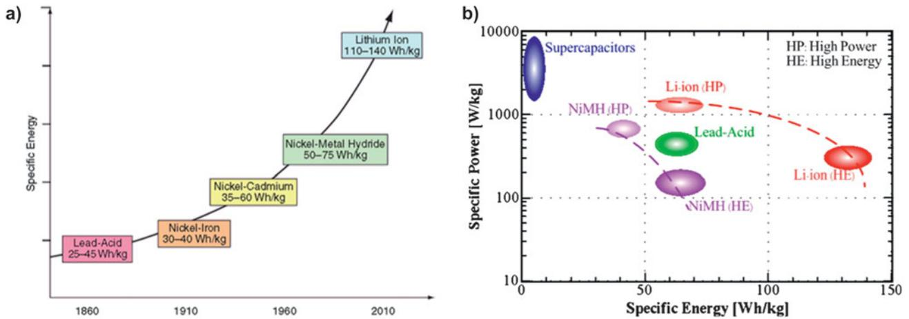
**Figure 2.** (a) Rapid advancements in increasing power density trend for batteries since the first lead-acid batteries were introduced in the mid-19th century<sup>42</sup>; and (b) specific power versus specific energy of modern storage devices: supercapacitor, lead-acid, NiMH, and Li-ion battery technology.<sup>43</sup>
