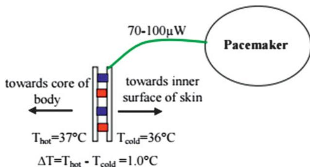
**Figure 4.** Schematic of a thermoelectric module showing the module attached to a pacemaker as an energy supplement to extend the lifetime of the pacemaker battery. The diagram demonstrates the approximate temperature difference available in the body. Source: Ref. 54.
